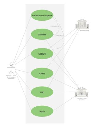
Credit Card Processing System UML Diagram. This sample shows the Use Case Diagram of the credit card processing system. You can see how the payment by credit card occurs. This sample can be used by the bank, financial enterprises, for understanding the work of the credit card processing system at the projecting the banking systems.
