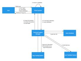
UML Collaboration Diagram depicts the interactions between objects or parts in terms of sequenced messages and describes both the static structure and dynamic behavior of a system.
