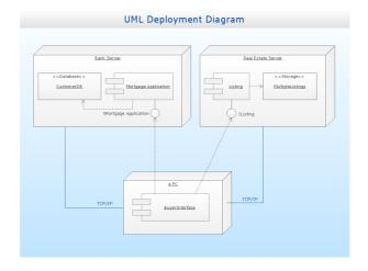
UML Deployment Diagram depicts the physical deployment of artifacts on nodes (nodes are the existing hardware components, artifacts are the software components running on each node); and how the different pieces are connected. Use ConceptDraw PRO with UML deployment diagram templates, samples and stencil library from Rapid UML solution to model the physical deployment of artifacts on nodes of your software system.
