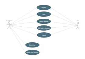
This sample was created in ConceptDraw PRO diagramming and vector drawing software using the UML Use Case Diagram library of the Rapid UML Solution from the Software Development area of ConceptDraw Solution Park. This sample shows the types of user's interactions with the system and is used at the registration and working with the database system.
