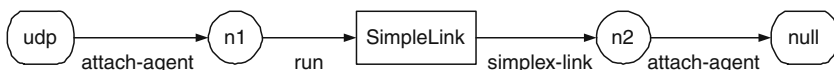
Fig. 7.4. A two-node network with a uni-directional link and the instprocs of class Simulator .
