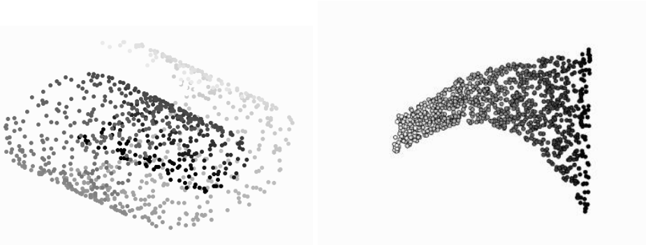
FIGURE 6.13 A common example used to demonstrate LLE is the swissroll dataset shown on the left. To produce a useful 2D representation of this data requires unrolling the data, which the LLE does successfully, as is shown on the right. The shades are used to identify neighbouring points, and do not have any other purpose.
