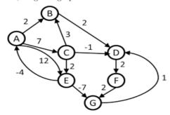
(a) Even though the graph has negative weight edges, step through Dijkstra's algorithm to calculate supposedly shortest paths from A to every other vertex. Show your steps in the table below. Cross out old values and write in new ones, from left to right within each cell, as the algorithm proceeds. Also list the vertices in the order which you marked them known.
